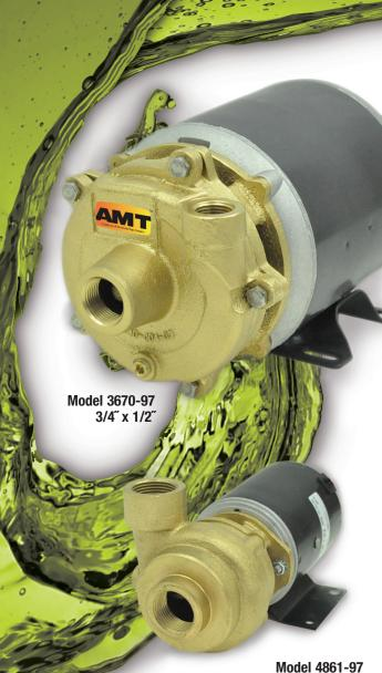
The AMT Model 3670-97 Naval Bronze Straight Centrifugal pump is designed for low pressure salt water wash down and recirculating applications. The pump has been sized for salt water (1.03 specific gravity) and feature provisions for the installation of a seal wash, front drain plug and pull-from-rear design. The pump is powered by a 1725 PM, 115 VAC, 1/4 HP motor.
