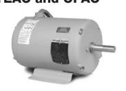
Features: TEAO design prevents entrance of rodents, insects and other foreign matter. High full load efficiency for reduced operating cost. No mechanical switch to wear. No noise and vibration from regeneration. Less sensitive to voltage variations. Soft start. Thermostats. Epoxy paint. 1.00 Service Factor. Class F insulation.
