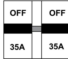
Figure 25. Main Circuit Breaker (OFF)
