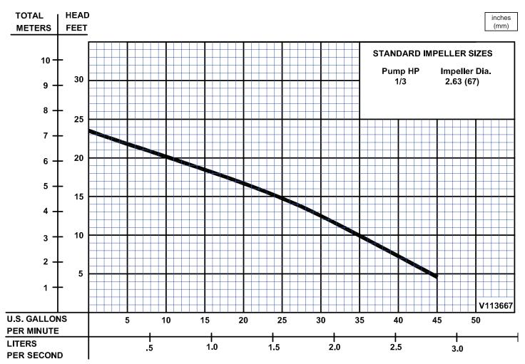
Testing is performed with water, specific gravity 1.0 @ 68º F @ (20°C), other fluids may vary performance
